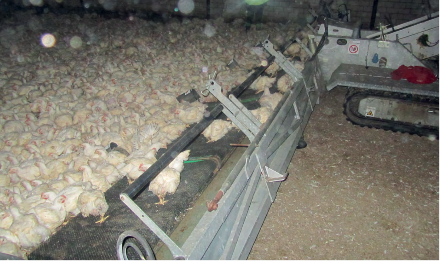
Figure 2.1 | Chicken harvester – catching equipment – with a system of conveyor belts picking up the birds from the litter floor, moving them to the centre of the harvester, and loading them into transportation crates (Jacobs, 2016).
